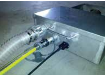
Easy push-in connections for LPG and power
